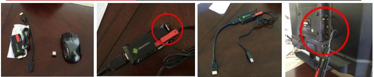
Connect the Mouse's USB piece to the end of the Device USB port / Slide the Red Antenna out / Connect the HDMI side of the device to the TV's HDMI1 Port / Connect the USB Side of the Device to the TV's USB Port
